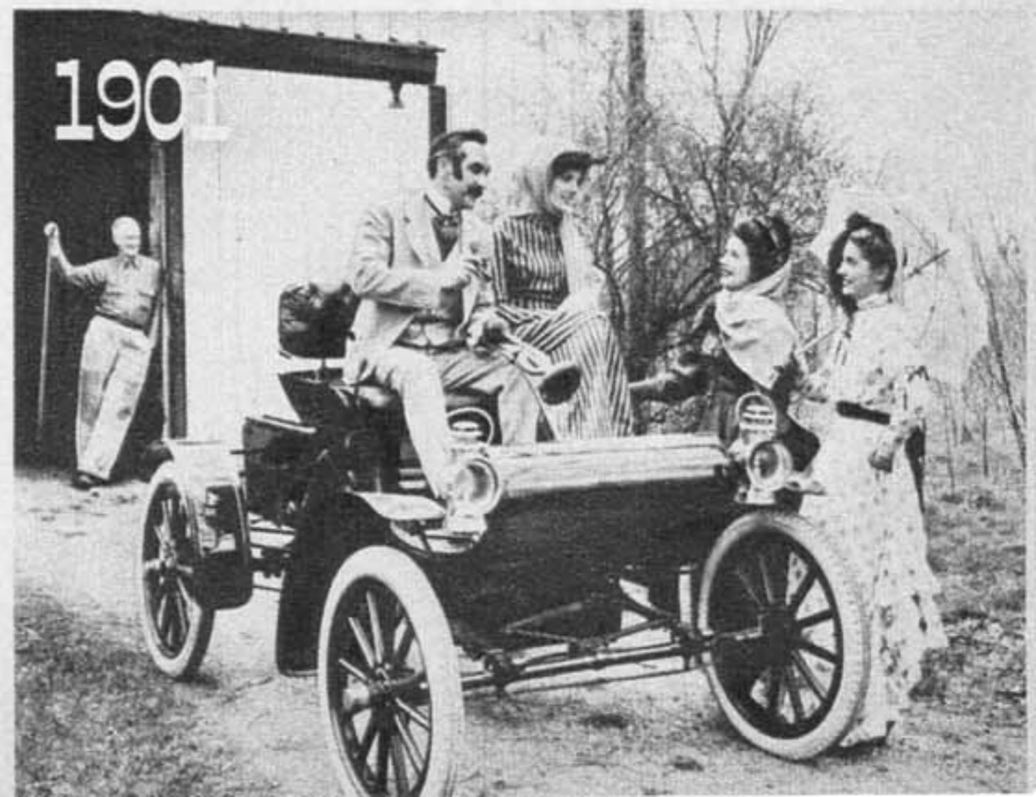
The earliest Curved Dash model (above) had a single-cylinder, watercooled engine of seven hp which propelled the car at 20 mph. Gas and water tanks held five gallons each. Folding top was extra.
