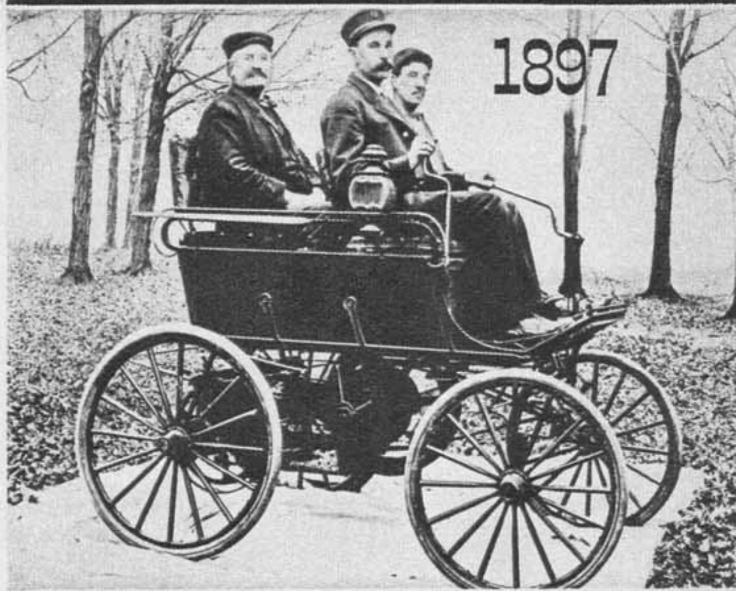
The first Olds auto (above) was built in a small shop, with help of Frank Clark. Speed was 10 mph, from a 9 hp engine with an oversized flywheel. Not for three years was the name Oldsmobile used.
