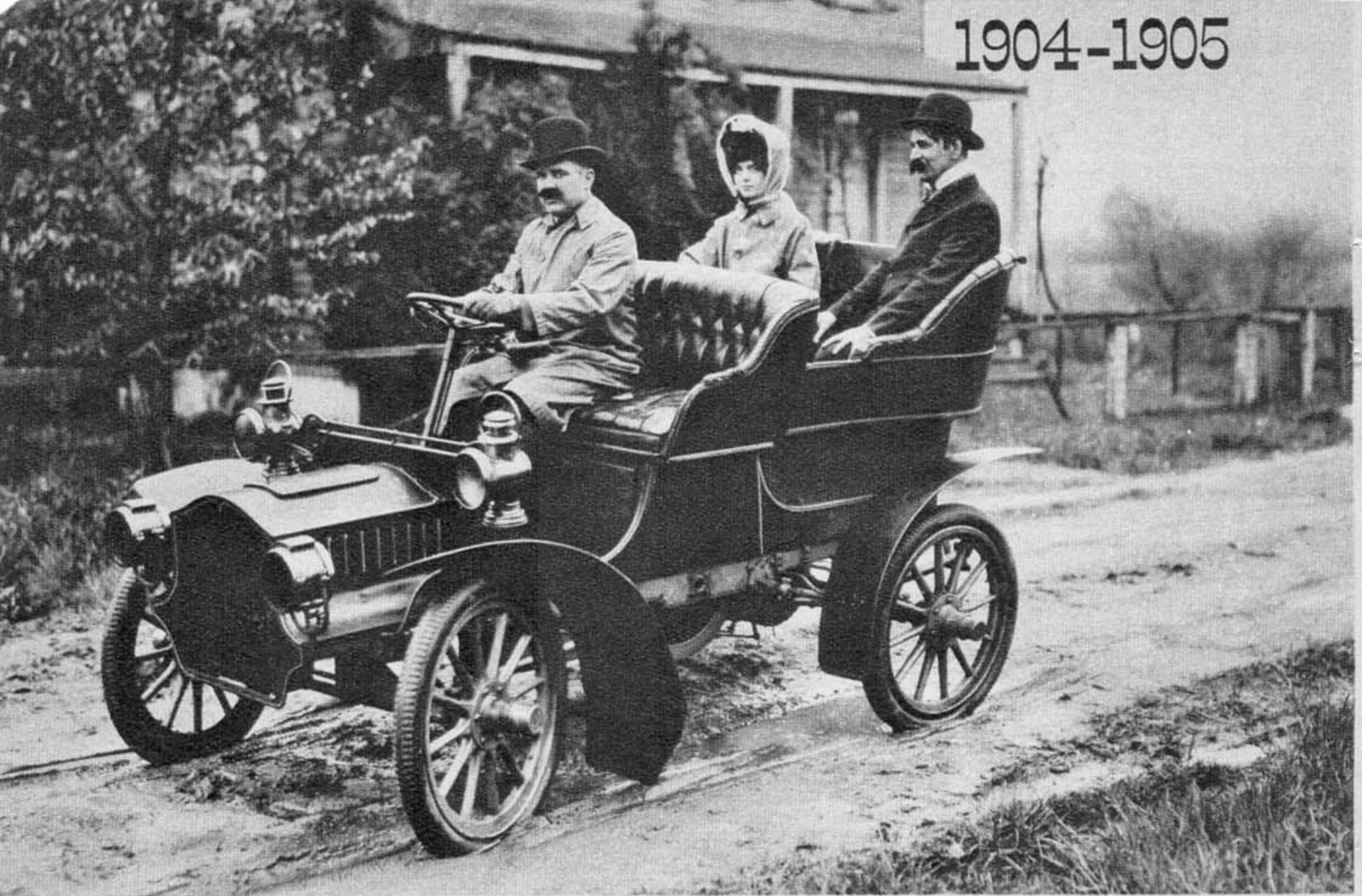
Mustachios were popular at the same time as this Model B Cadillac. It was a one-cylinder 8 hp. job.
