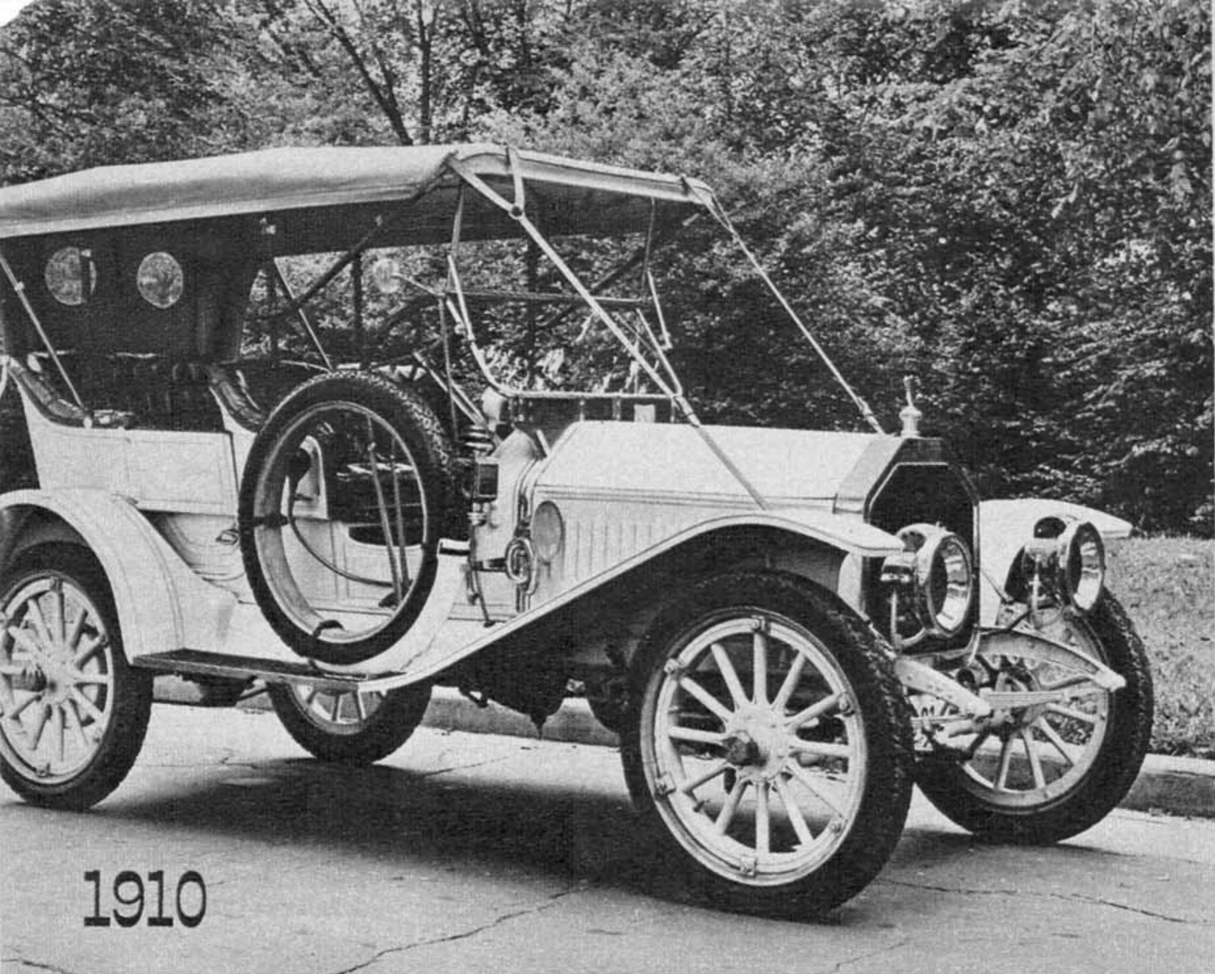
This Model 16 touring car (above) carried four passengers and sold at $1,750. It had a four-cylinder 30 hp engine, 112-inch wheelbase. Produced: 2,252 units.
